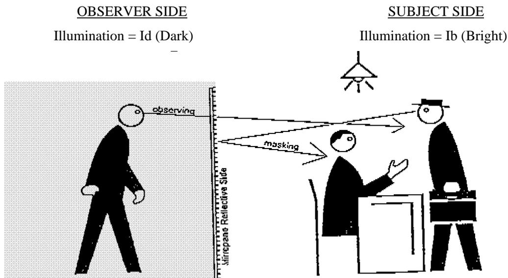
The transparent mirror must be installed with the reflective surface (coated side) towards the subject side. Note also that this side must have the higher level of illumination. The optical ratios are defined as follows:
